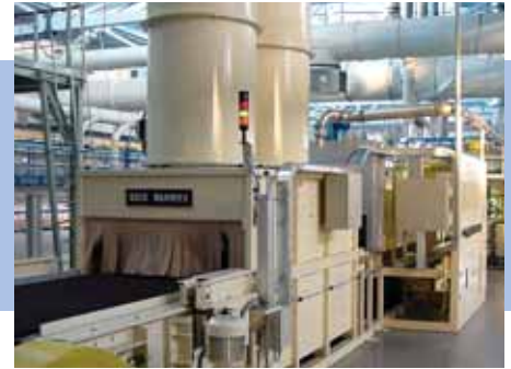
CAB Brazing Furnace System
