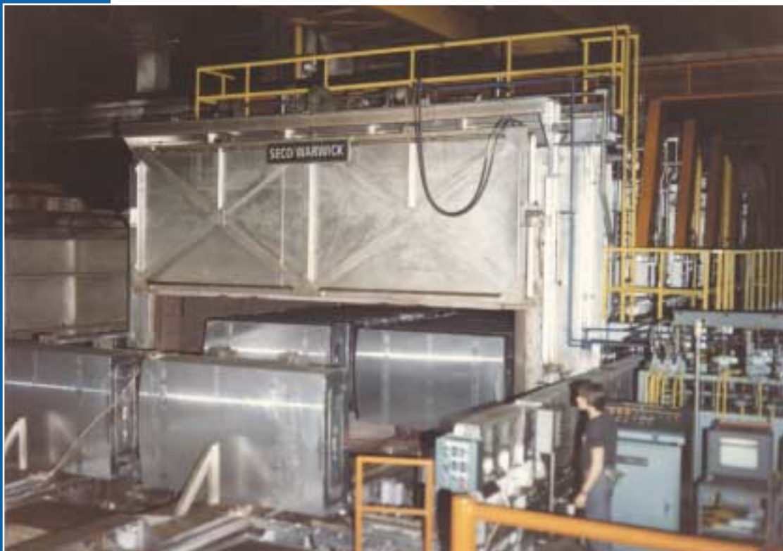
Single or double row design pusher furnace
