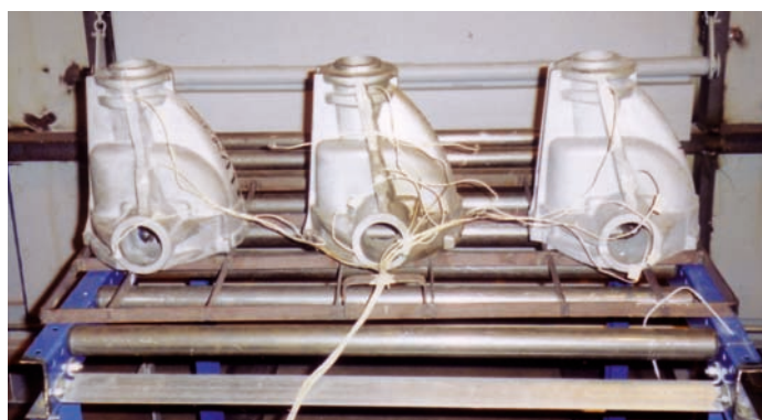
Fig. 5 Test load of Castings
