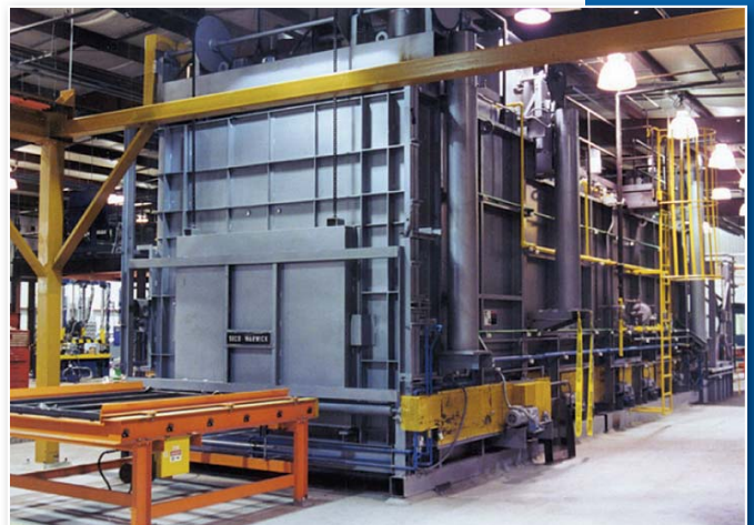
Solution Heat Treat Furnace, front view.
