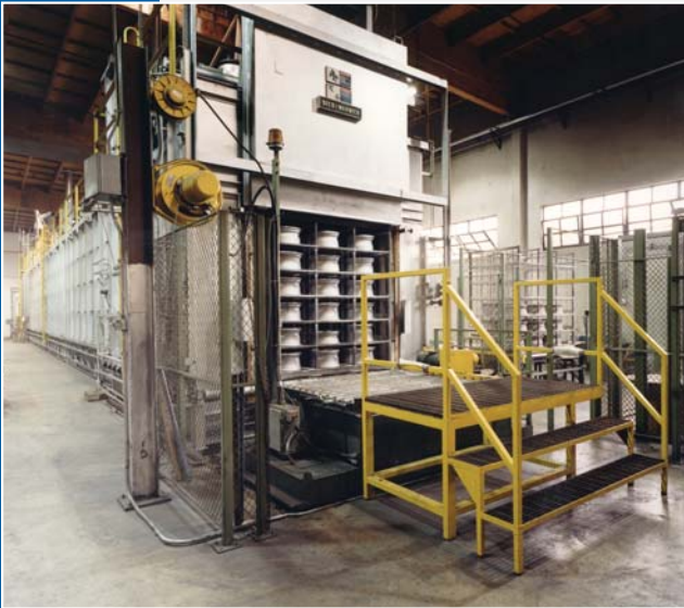
Fully automated solution heat treat and aging system for automotive wheels
