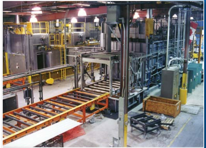
Solution Heat Treat Furnace and age oven system for aluminum differential carrier castings
