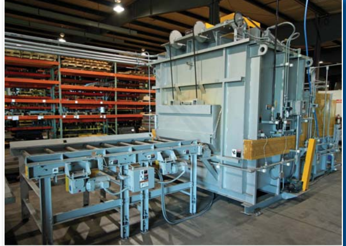
Solution Heat Treat Furnace equipped with Jet Impingement Technology for aluminum stamping application
