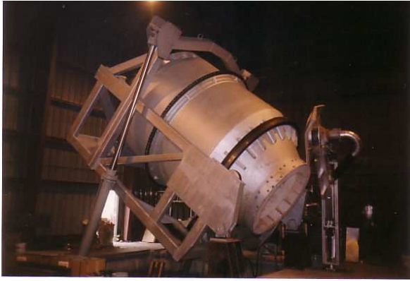
Photo 6: Scrap Manager™ Tilting Rotary Furnace
