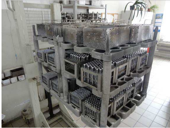
Fig. 12. Tooling, packeting and segregation of workpieces
