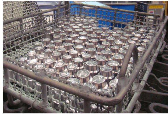
Fig. 4. Mint dies in a basket after heat treatment
