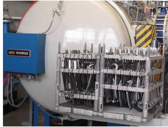
Fig. 5. Packing of surgical tools in a workload
