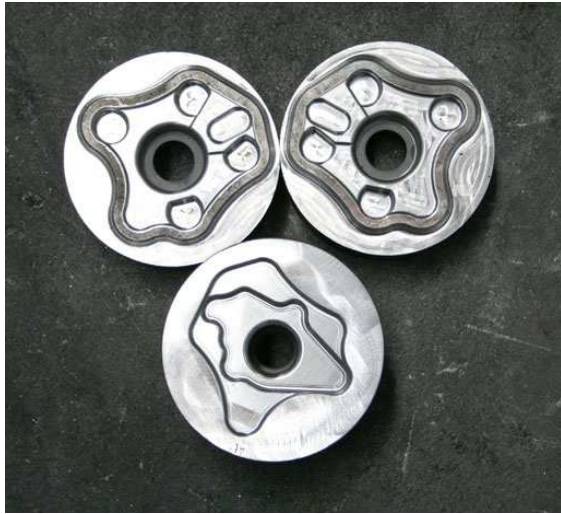
Fig. 7. Examples of hot forging die inserts made of WCL steel
