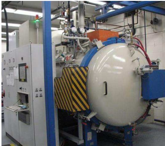
Fig. 3. Vacuum furnace for toughening of dies and punches, SECO/WARWICK type 15.0VPT-4025/24HV
