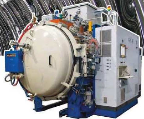
Fig. 1. Furnace 25VPT4035/36 (24 x 24 x 36 inch) 800-kg charge capacity
