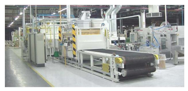
Figure 3 Mesh belt brazing system
