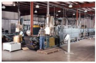
production line operations accepting parts Figure 1 - Mesh Belt Conveyor systems used for ready for heat processing and discharging copper brazing in commercial heat treat facility
