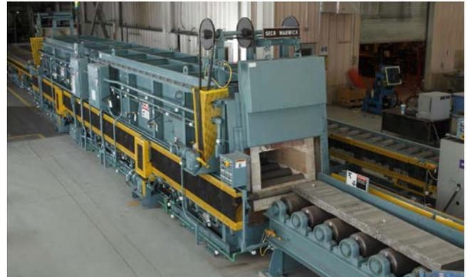
Figure 1 Roller hearth for zirconium and hafnium billets
