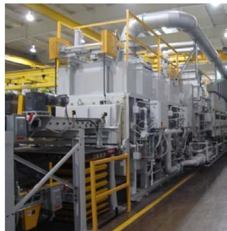
Figure 2 Roller Hearth System for motor lamination annealing
