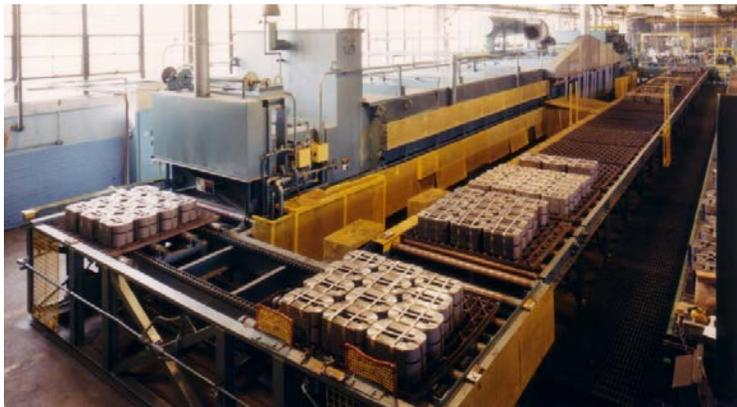
Figure 6 Two configurations (above and below) of transformer core annealing systems with automatic loading and unloading
