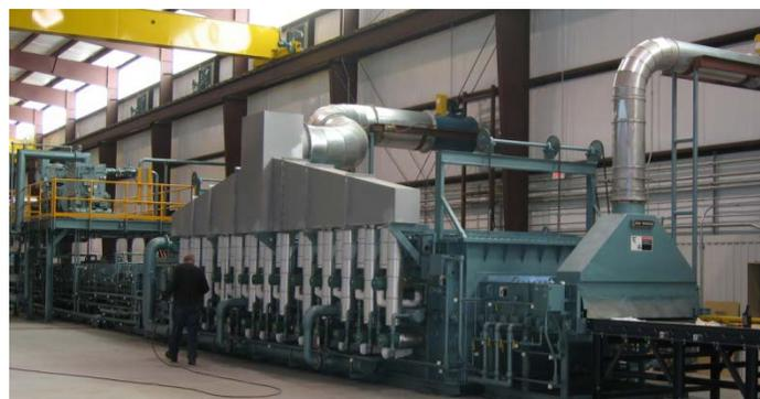
Figure 4 Roller Hearth Furnace System for tube and pipe annealing with custom engineered additions to accommodate customer space limitations
