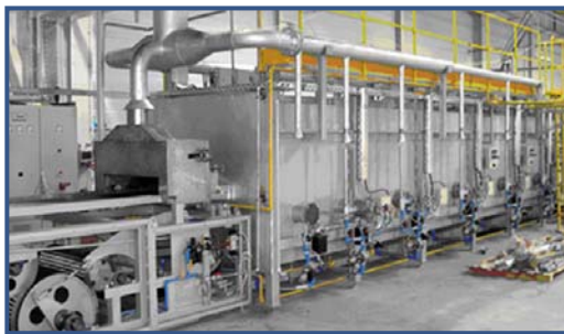
Mesh belt furnace lines for nitrocarburizing, hardening and tempering of small hydraulic components
