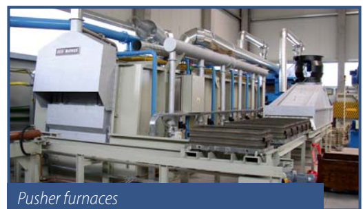
Roller hearth furnace line for heating-up before quenching on press, washing and tempering of bearing rings
