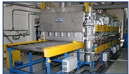
Roller hearth furnace line for heating-up before quenching on press, washing and tempering of bearing rings
