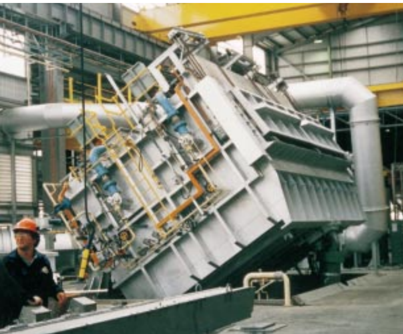
▼ Tilting reverb melter/holder with a capacity of 38 metric tons
