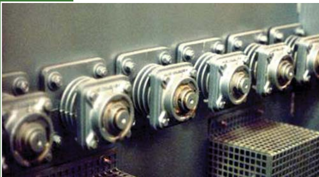
External, air-cooled bearings are not subject to thermal cycling and can be designed for maximum operation life
