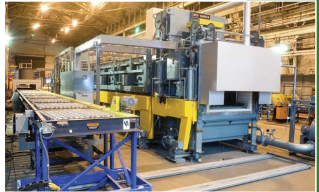
Roller hearth transformer core annealing system with fully automated temperature and atmosphere control system
