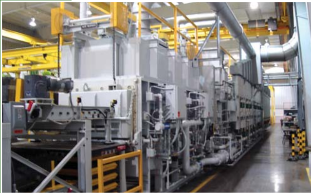
Continuous roller hearth furnace line for motor laminations with custom-designed tray handling system to increase production capacity
