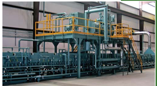
Roller hearth for continuous tube annealing with atmosphere system mounted over the furnace line to conserve plant floor space
