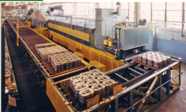
Transformer core annealing furnace with return conveyor system and cross transfer for ease of loading and unloading product
