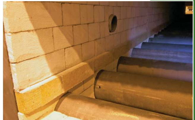
Hard brick rub rails protect both the furnace walls and product while traveling through the furnace
