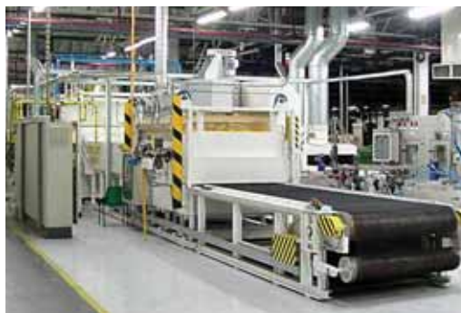
Mesh Belt Brazing Furnace
