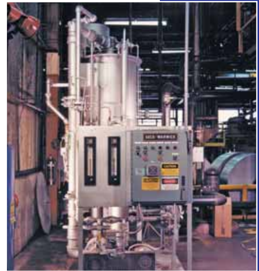
Exogas® Direct Chill Generator for large volume production of exothermic gas, typically for aluminum furnace applications
