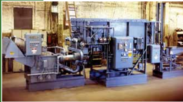
Standard 500 pound per hour Rotary Retort Furnace with metering loader and Whirl-A-Way quench.
