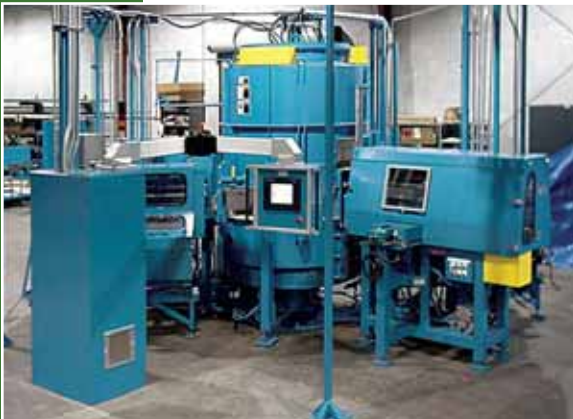
Rotary Hearth Furnace
