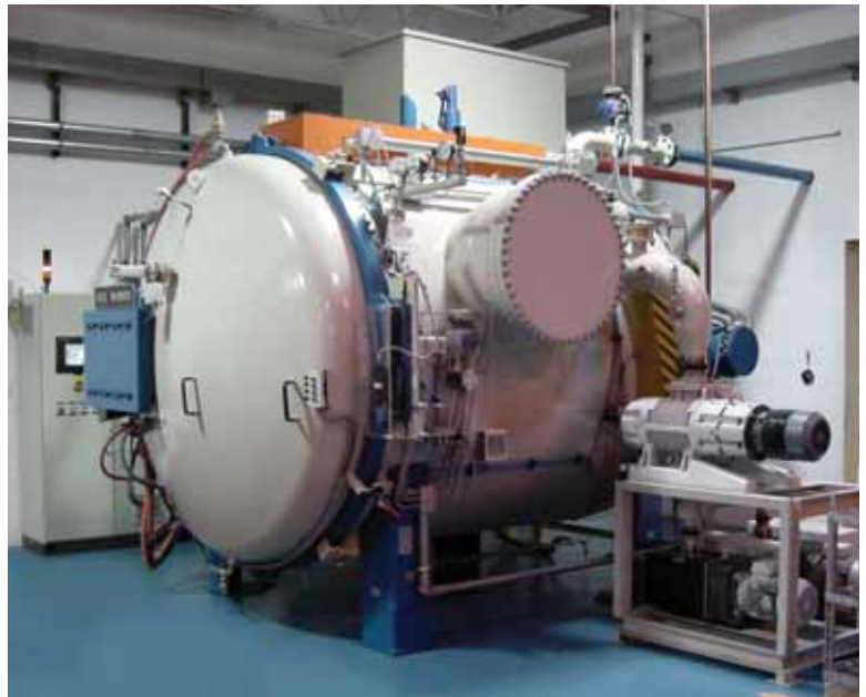
10 BAR HPQ used specifically for vacuum heat treatment of H-13 die material
