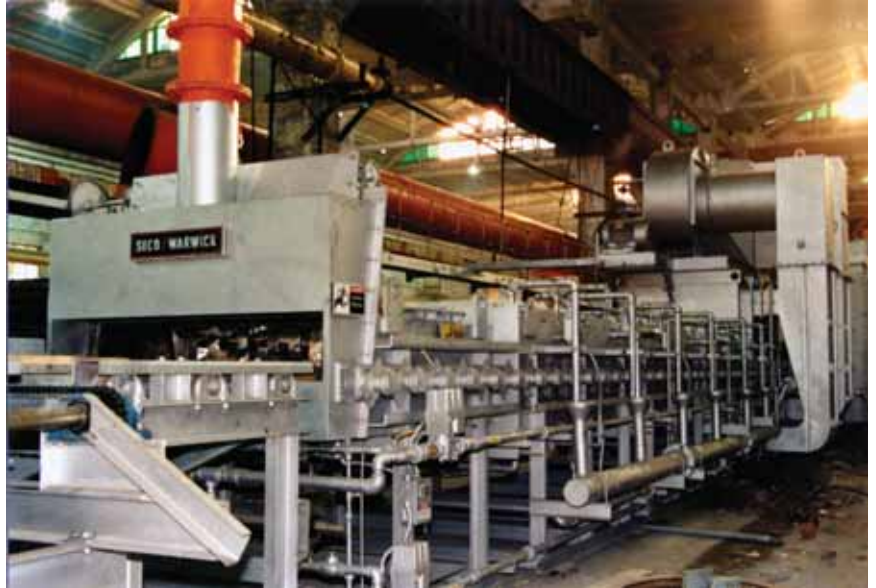
15,000 pounds (6,800 kg) per hour continuous roller hearth furnace line for carbon steel and alloy tubing
