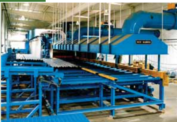
10,000 pounds (4,540 kg) per hour roller hearth for stainless steel tubing
