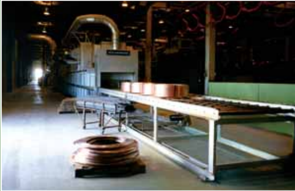
5,000 pounds (2,270 kg) per hour continuous roller hearth for wound copper tubing
