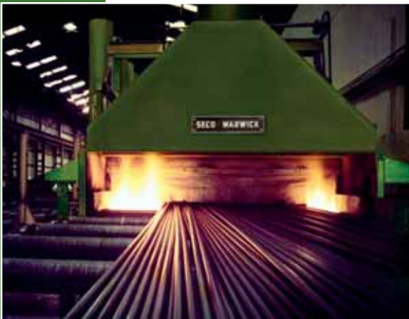
12,000 pounds (5,440 kg) per hour continuous tube annealer - carbon steel pipe
