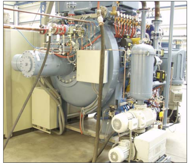
a) Fig. 1 The vacuum carburizing devices: special two-chamber furnace with cold chamber “ColdCam” (a) and the Universal HPQ™ vacuum furnace with carburizing option (b)
