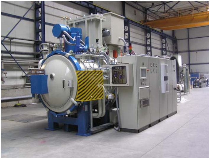
a) Fig. 1 The vacuum carburizing devices: special two-chamber furnace with cold chamber “ColdCam” (a) and the Universal HPQ™ vacuum furnace with carburizing option (b)
