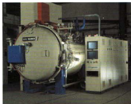
Typical HPQ furnace with 16-bar gas quenching.
