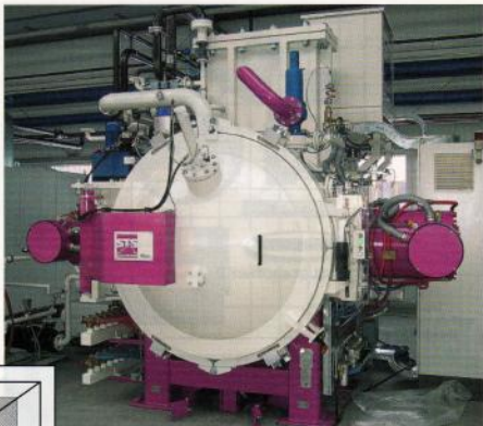
Fig. 9 - Double-chamber 24 x 24 x 36 in. furnace with 20-bar quenching.
