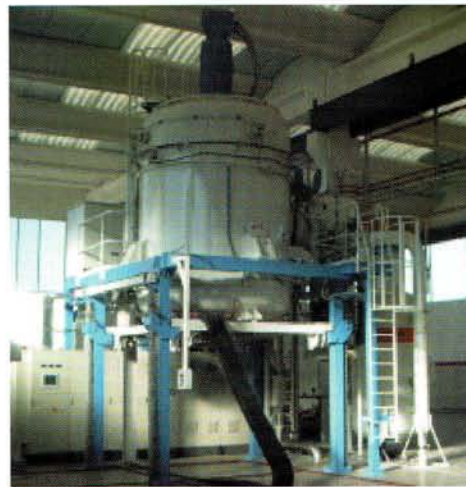
Fig. 5 — Elevator furnace (72 in. diam. × 72 in. high) with axial/radial quenching.
