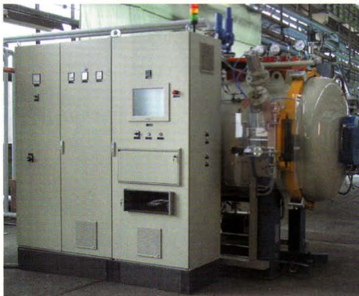
Fig. 7 — HPQ furnace with 16 × 16 × 24 in. work chamber.
