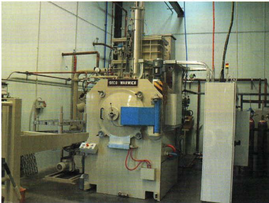
Fig. 12 — Double- chamber oil-quench furnaces 18 × 20 × 24 in. (top) and 30 × 24 × 48 in. (right) work chambers.
