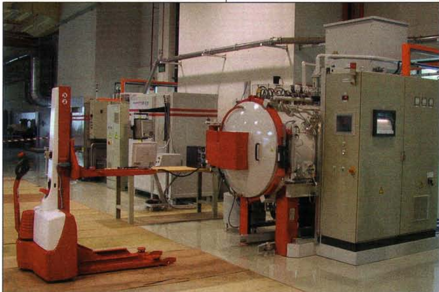
Representative vacuum brazing furnace system with front end parts loader (left) and view of an all metal hot zone (right).
