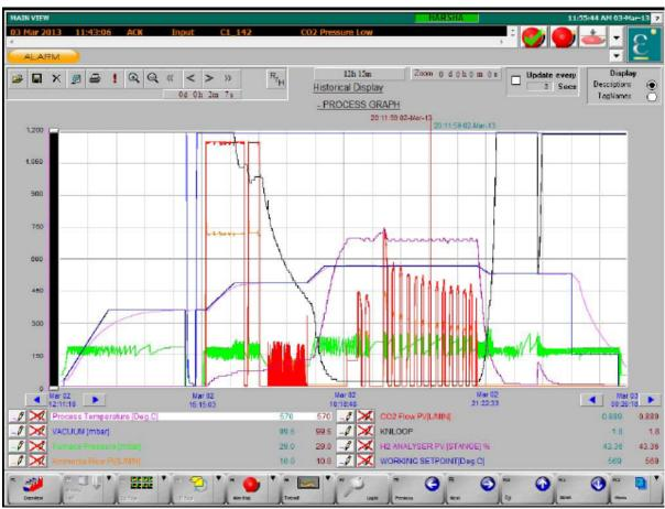
The furnace control system employs cascade based temperature control system to regulate the furnace temperature very closely to meet stringent AMS 2750 D requirements of the customer.
