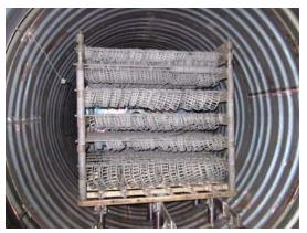
The furnace is a horizontal retort furnace with facilities to do nitrocarburising of bearing cages by zero flow method.
