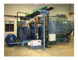
The furnace is equipped with vacuum system, gas control system, turbo cooling, atmosphere cooling system and post oxidation system to get material very uniform grey color and other tribological properties to meet the specifications of leading bearing manufacturers
