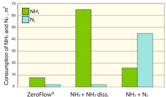
Comparison of consumption of NH<sub>3</sub> and N<sub>2</sub> in the traditional processes and ZeroFlow® during nitriding of wheels for wind power plants made from steel 31CrMoV9 (retort volume – 0.6 m<sup>3</sup>)
