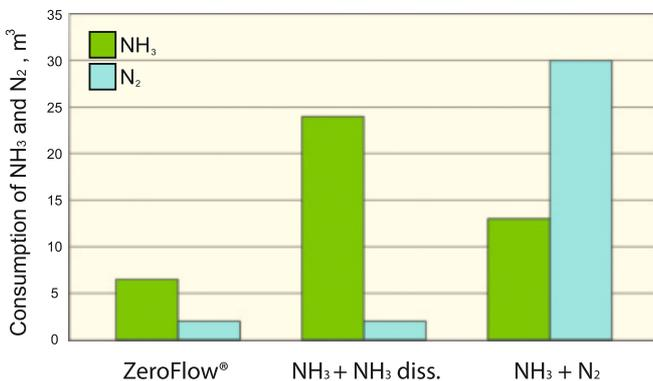
Comparison of consumption of NH<sub>3</sub> and N<sub>2</sub> in the traditional processes and ZeroFlow® during nitriding of a crankshaft made from steel 4340 (retort volume – 0.6 m<sup>3</sup>)
