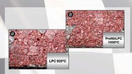
Case structure of steel 16MnCr5 depending on the applied technology:
