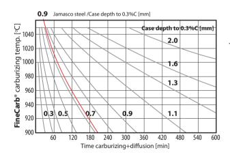
**FineCarb**<sup>®</sup> - The method of Carburizing Steel in an Oxygen Free Atmosphere Under Low Pressure
