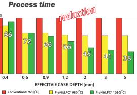
**<sup>4</sup>** Total process time reduction depending on the effective case depth & applied technology (Conventional, PreNitLPC<sup>®</sup>)
