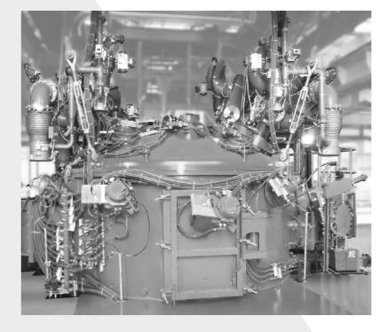
A Retech Electron Beam (EB) furnace utilizes the ease of use and low maintenance of Von Ardenne guns to melt reactive and refractory metals in a sealed vacuum chamber.
