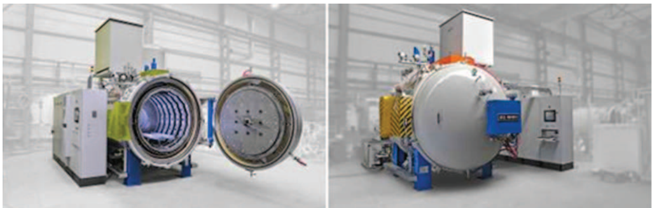
6 Horizontal vacuum furnaces for tool treatment (VECTOR vacuum furnaces from SECO/WARWICK, size 900/800/1200 \text{ mm} and 1200/1200/1800 \text{ mm} , 15 bar quench)
