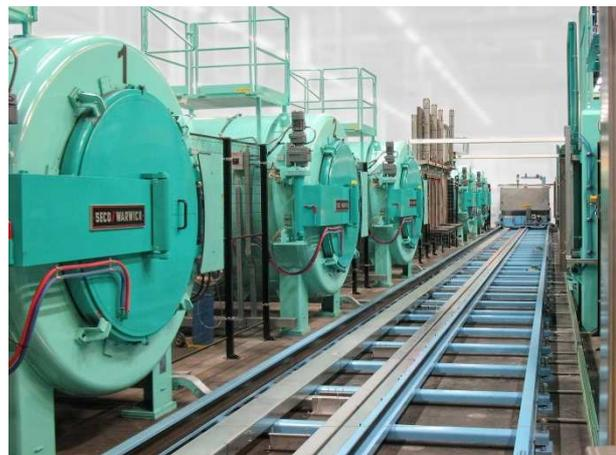
*Fig. 1 Picture of the nitrocarburizing system at work*
