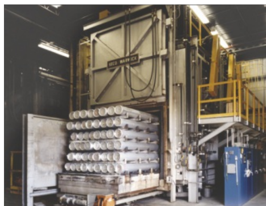
Batch style furnace with car
