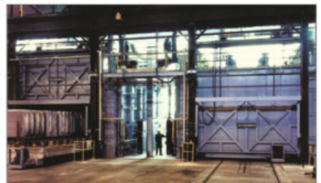
Car bottom ingot soaking for billet heating
