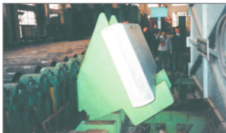
Discharge end with ingot down-ender and mill roll table
