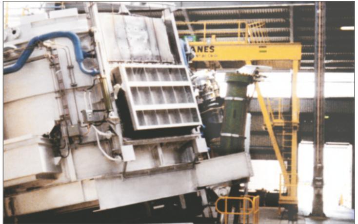
*Round melting furnace in the tilting position*
