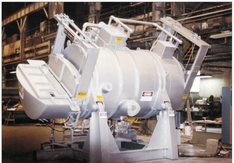
*Tilting barrel furnace applications*
