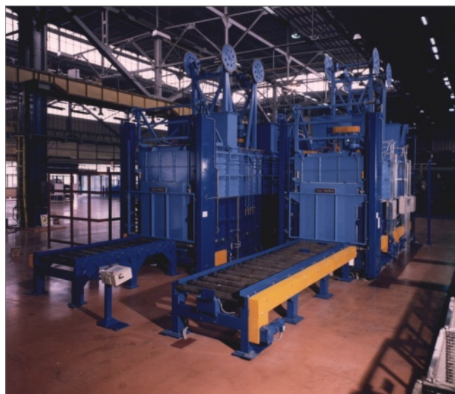
Solution heat treat furnace, front view
