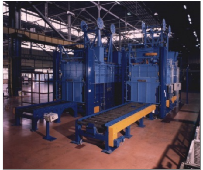
Solution heat treat furnace, front view
