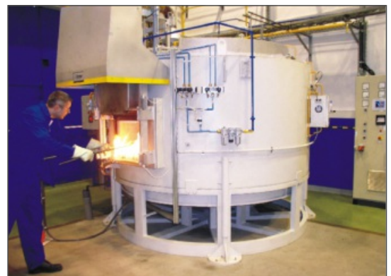
Furnaces with manual loading system
