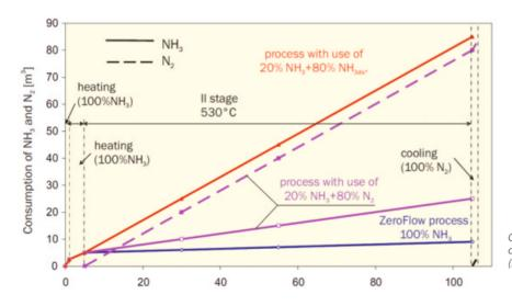
Consumption of NH3 and N2 in processes with use of double-component atmospheres (NH3 + NH3 diss. and NH3 + N2 ) and ZeroFlow<sup>®</sup>
