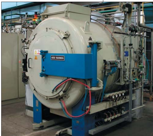
Horizontal furnace for nitriding using ZeroFlow process. Photo courtesy of Seco/Warwick Group, Swiebodzin, Poland.
