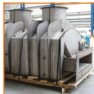
Convection Muffle US Patent #5,271,545
