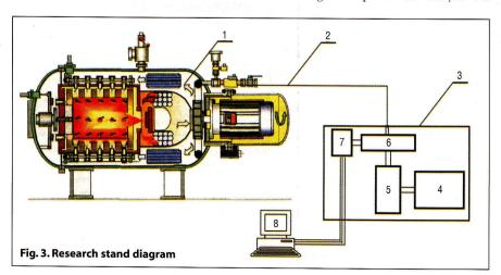
mass spectrometer (3). Particles were ionized in the ionization chamber (6) inside the spectrometer, detected by a detector (7) and analyzed in the quadruple analyzer (5), the results converted into a measurable signal registered by the computer (8).
