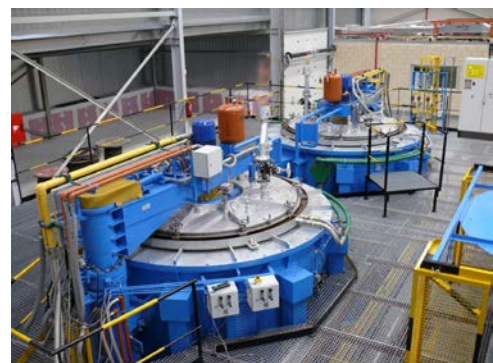
Pit Furnaces are an ideal choice for nitriding applications
