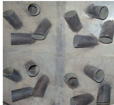
Fig. 1: Vortex nozzles system
