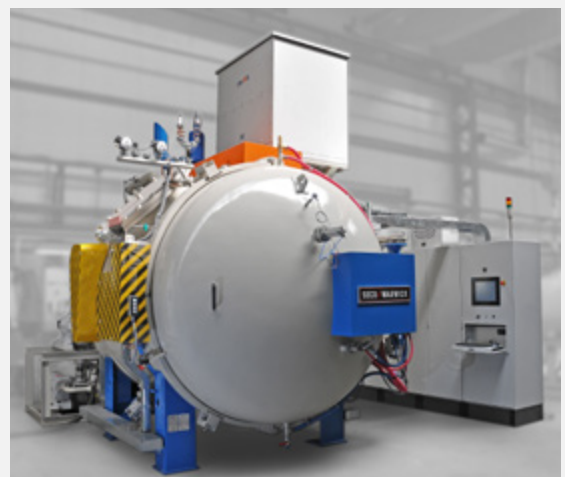
Fig. 4: Horizontal vacuum furnaces VECTOR line (Seco/Warwick) size 900/800/1,200 mm, 15 bar.
