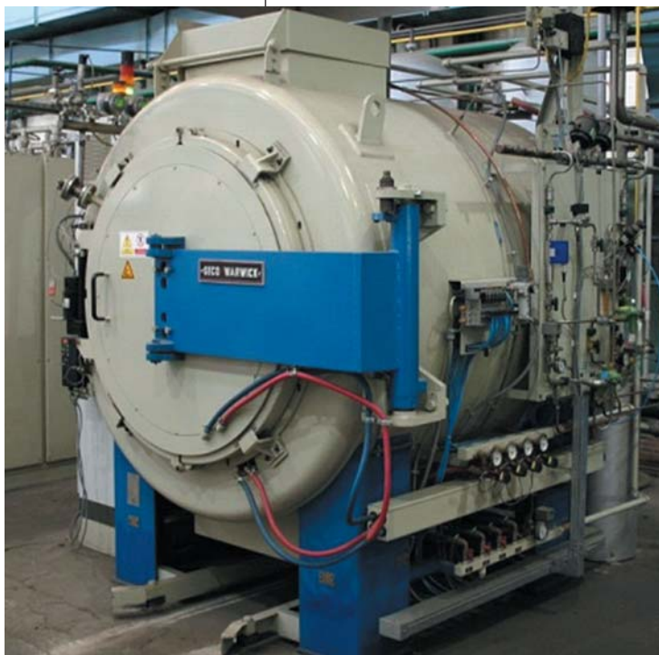
Fig. 1 — Horizontal furnace for nitriding using ZeroFlow process.
