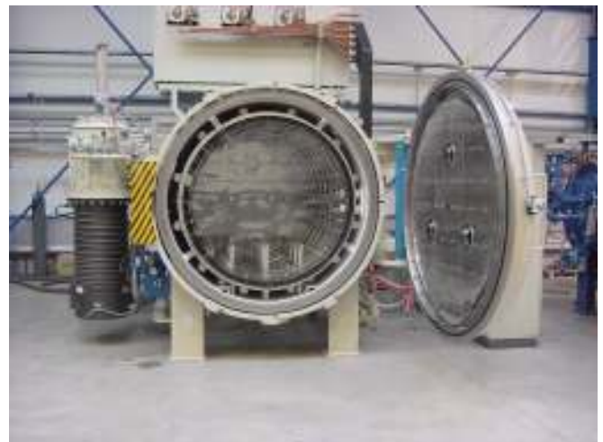
Figure 8 Vacuum Brazing Furnace with All Metal Hot Zone
