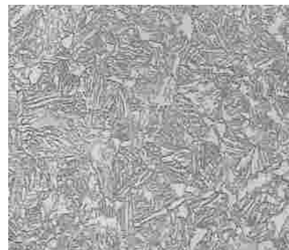
Pict.3: 16MnCr5 LPC - the core 263 HV10 magn. 500x
