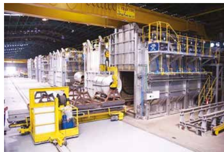
Seco/Warwick vortex coil annealing installation.
