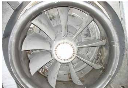
Specially developed semi-axial fan.
