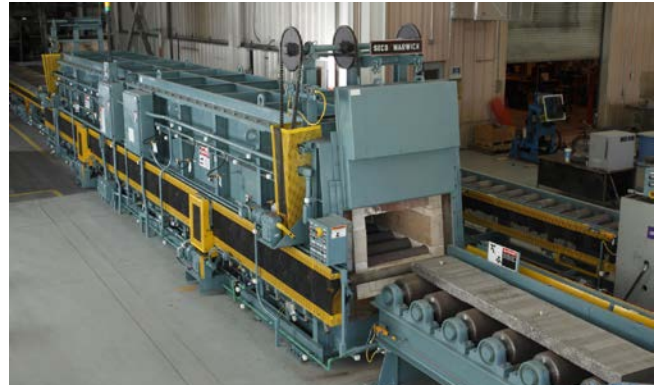
Figure 1 Roller hearth furnace for billets & plates
