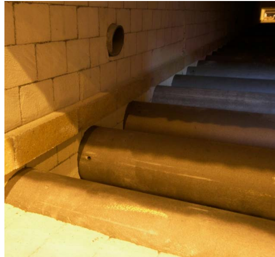
Figure 5 Furnace rub rails protect both the furnace walls and product while traveling through the furnace
