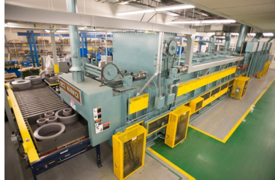
Figure 3 Continuous transformer core annealing
