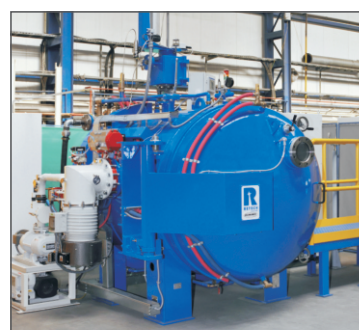
Pic 2. „Batch type VIM furnace for pilot production“
