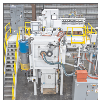
Pic 3. „50 kg EQ for production of turbine blades“
