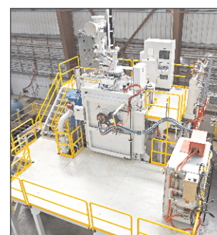
Pic 4. „100kg EQ for production of turbine blades“
