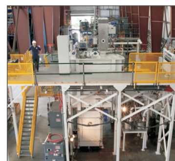
Pic 5. „200 kg EQ/DS/.S.C. VIM for production of large turbine blades“
