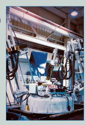
Rototrode® technology can be applied to tilt-pour crucibles for parts casting, static crucibles for producing metal ingots and bottom-pour crucibles for powder production. Our unique system enhances complete alloying and melting of materials by producing and holding hotter pool temperatures for precision controlled periods of time. This also allows most forms of scrap to be readily upgraded to ingot quality, increasing the customer's bottom line.
