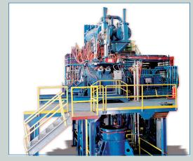
melting is its ability to maintain alloy composition over a wide band of complex alloys. Processing in an inert gas environment prevents the loss of volatile alloying elements during melting, thus reducing the need to adjust the alloy empirically. Retech Plasma melting systems are the right choice for producing high-performance, complex alloys with zero defects.
