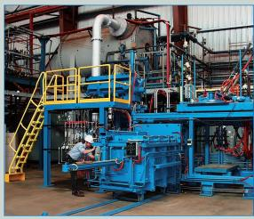
More types of waste can be simultaneously treated in our patented plasma arc melter than in any other process or technology; Retech's plasma systems can accept multiple streams of a wide range of solids, slurries, liquids and gases.
