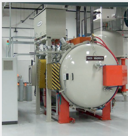
Fig. 4: High temperature vacuum furnace with high pressure quench
