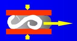
Convection is the transfer and exchange of heat, due to the mixing motion and movement of a fluid.
