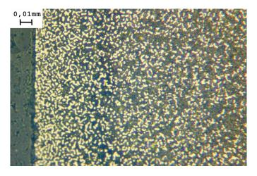
Figure 6b – Comparison of the CSB-50 NIL steel structure obtained after successive stages of the heat treatment under 0464 process
