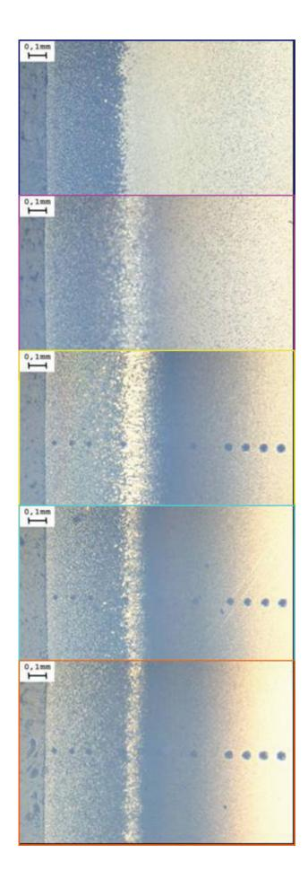
Figure 6a – Comparison of the CSB-50 NIL steel structure obtained after successive stages of the heat treatment under 0464 process
