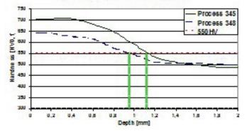
Figure 4 – Distribution of hardness HV 0.1 on the cross section of the hardened layer of Ferrium C61 specimens, thermochemical treated in the processes 345 and 348
