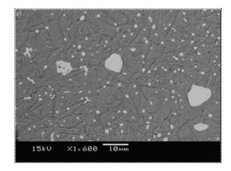
Figure 9b. Case, after hardening from  $1175^{\circ}C$  (2147°F) and double tempering at  $560^{\circ}C$  (1040°F) – white inclusions of
