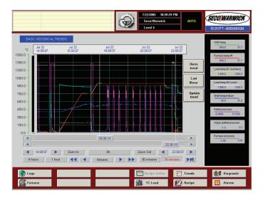
Figure 2. FineCarb low pressure carburizing process cycle
