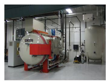
Figure 1. Vacuum furnace, LPC + HPGQ Type 15.0 VPT-4050/48N
