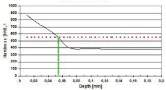
Figure 10- Hardness distribution on the cross section of the carburized layer of the steel X5CrNiMo17-12-2
