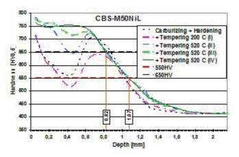
Figure 7- Distribution of the case micro-hardness HV 0,5 of the CSB50 NIL steel after the 0464 process
