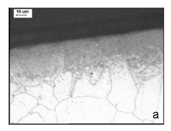
Figure 11a –Photographs of the microstructure of the carburized layer of the steel X5CrNiMo17-12-2. Case after 2 min carburizing at  $1050^{\circ}C$  (1922°F)
