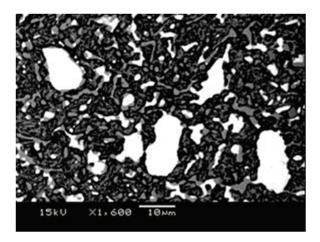
Figure 9a.. Microstructure of the case of the screw-tap,  $\Phi 8 mm (0.315")$ , 6-5-2 steel.
