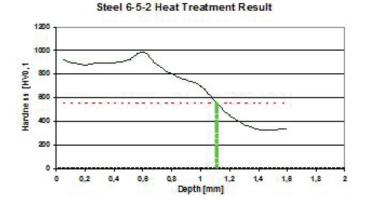
Figure 8 – Case hardness profile on the cross section of the screw-tap,  $\Phi 8 \text{ mm} (0.315^{\circ})$ , 6-5-2 steel.
