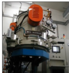
Sintering of SiC 2300°C
